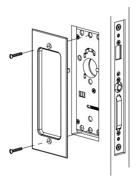
Secure both inside and outside plates using machine screws (provided)
